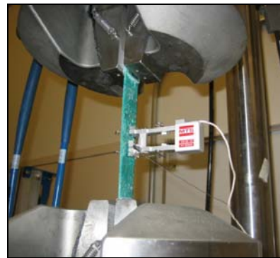
Figure 7 - Coupon test setup
