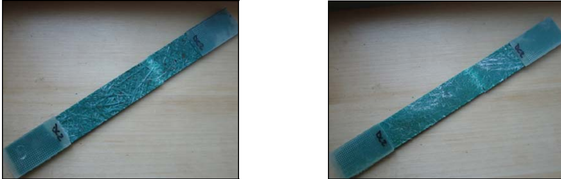
Figure 8 - Typical tensile failure of specimens: left (front side), right (back side)
